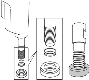
**NOTICE!** The friction ring is used to prevent damage on the shaft and the gear box during the dismantling of the drill bit.
